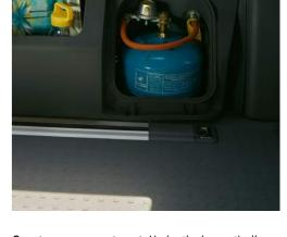
Gas storage compartment. Under the hermetically sealed cover, an optional 1.8 kg Campingaz gas cylinder <sup>1</sup> can be securely attached to straps and connected to the gas hose.
